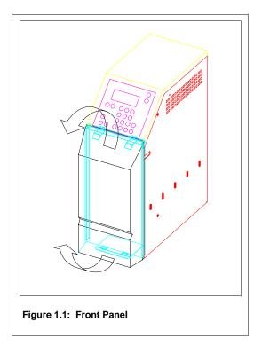
it in place. Press up on the bottom of the cover and swing it out to free it from the chassis.
