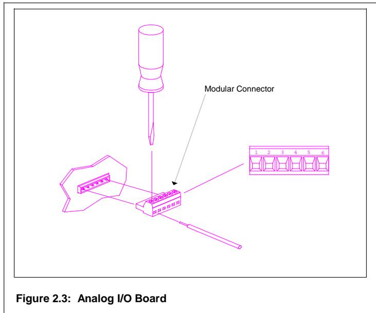
**Figure 2.3: Analog I/O Board**
