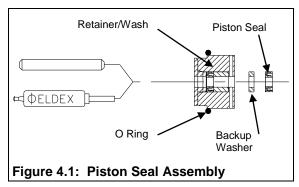
scratch the walls of the piston seal gland in the liquid cylinder with the tool/dowel pin.
