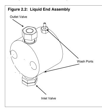
Optos stainless steel pumps with  $\frac{1}{4}$ " pistons use 1/8" Swagelok® fittings on the inlet and outlet valves and use 1/8" tubing (not supplied) and require a 7/16" wrench to tighten the fittings and a  $\frac{1}{2}$ " wrench to tight the valves.
