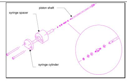
Figure 1: Syringe Cylinder and Piston
