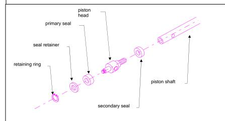
Figure 2: Syringe Piston Detail
