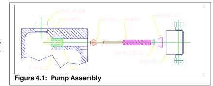
used to remove the seals). If you are using the 1/8" installation tool, hook the existing seals and remove and discard both the washer and the seal. If you are using the  $\frac{1}{4}$ " dowel pin, rock the dowel pin back and forth gently, and remove and discard both the washer and seal. Do not scratch the walls of the piston seal gland in the liquid cylinder with the tool/dowel pin.
