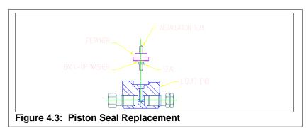
spring side down (the seal will generally "snap" onto the tool). Position the parts on the tool as shown in Figure 4.2. Insert the tool into the liquid end bore as shown in Figure 4.3. **CAUTION:** The open side of the seal (side revealing the spring) should face the closed (fluid side) end of the liquid end.
