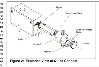
8. Finger tighten the assembly with the knob so the liquid end is against the pump body (two screw/knob assemblies are provided, you may wish to use the shorter one when the pump has a wash system installed).
