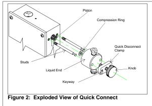
8. Finger tighten the assembly with the knob so the liquid end is against the pump body (two screw/knob assemblies are provided, you may wish to use the shorter one when the pump has a wash system installed).
